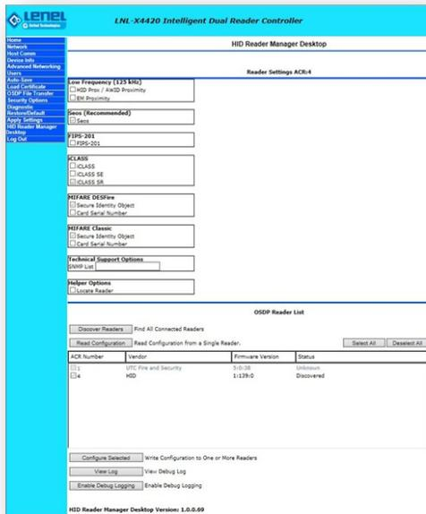
Figure 4: Changing Configuration (Turn Off Low Frequency)
